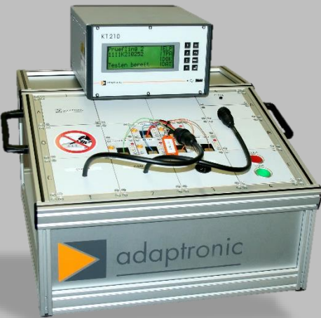
Test console PT 40 with wiring tester KT 210
