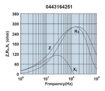
Impedance, reactance, and resistance vs. frequency.
