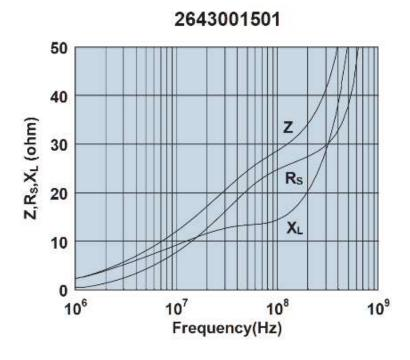
Impedance, reactance, and resistance vs. frequency.
