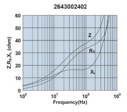
Impedance, reactance, and resistance vs. frequency.
