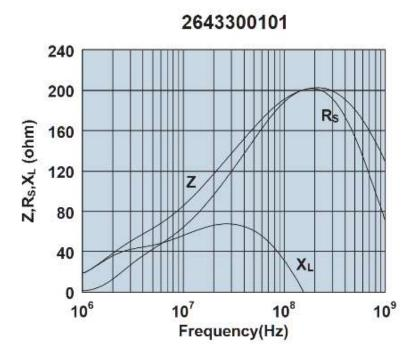
Impedance, reactance, and resistance vs. frequency.
