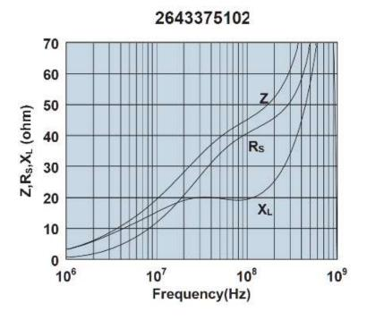
Impedance, reactance, and resistance vs. frequency.
