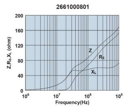
Impedance, reactance, and resistance vs. frequency.
