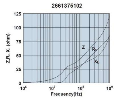
Impedance, reactance, and resistance vs. frequency.
