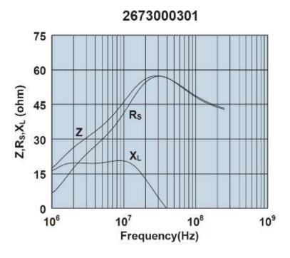
Impedance, reactance, and resistance vs. frequency.
