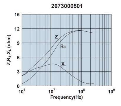
Impedance, reactance, and resistance vs. frequency.
