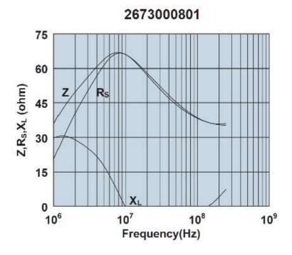
Impedance, reactance, and resistance vs. frequency.
