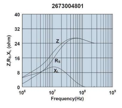
Impedance, reactance, and resistance vs. frequency.
