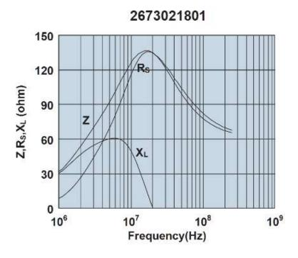
Impedance, reactance, and resistance vs. frequency.
