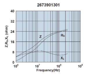
Impedance, reactance, and resistance vs. frequency.
