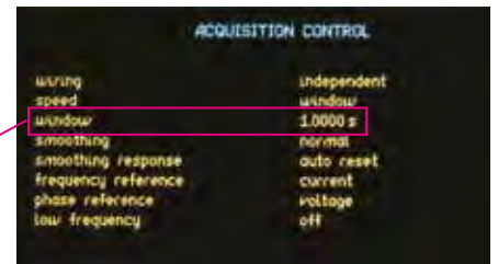
Example of setting the window, eg (50Hz set to 20ms)
