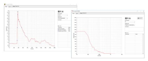
The transfer functions of all montena sensors and some other pulse measurement devices are preconfigured. The user has the possibility to add and edit additional components.
