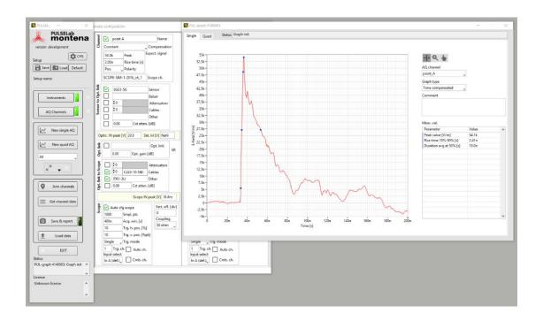
PULSELab improves the measurement accuracy by considering the transfer function of all devices used in the measurement chain (sensor, attenuators, cables, fibre optic link, etc.) and compensates the signals received by the oscilloscope to display the measured value in its own units. The correction factor of each component can be either a constant value or a frequency dependant transfer function.
