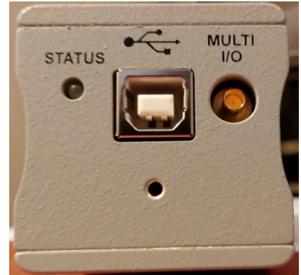
Figure 2.16 The 55 Series end panel showing the connectors and Status LED.
