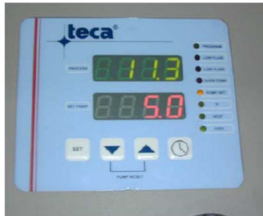
Figure 4.8 Pump is Primed Correctly
