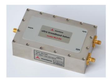
The BL3-5G balun can be used to measure differential signals, for instance produced by derivative electromagnetic free field sensors. The phase and amplitude balances are excellent and the frequency range is extremely wide. This allows faithful measurement of signals like pulses for instance. The shielding effectiveness of the device allows measurements in a disturbed environment. As the balun is passive and all the accesses are 50 ohm, it can be used in both directions.
