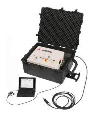
The portable generator **PPG-E1-1200** generates output current pulse according to MIL STD 188-125, E1. It has an internal impedance of >60 ohm and its charging between may be set between <5 kV and 80 kV. It delivers short circuit current pulses in the range of <50 A to 1200 A
