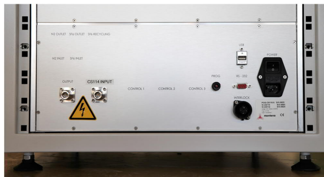
Figure 2 : signal output (on left side) on the generator's rear panel
