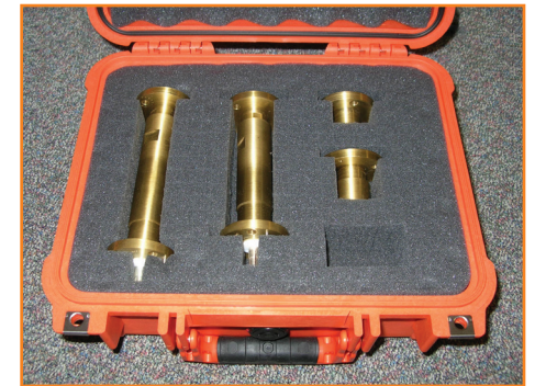
Figure 1 Mismatch Load Standards for 0.5 - 4.5 GHz
