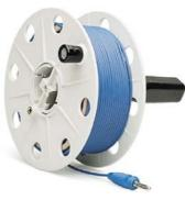
50 m measurement cable coiled onto a metal drum. Connection to the inside end of the cable is made possible with a socket integrated into the drum. The other end is equipped with a banana plug. The drum axle with handle can be removed for space saving storage. Cable resistance can be compensated for with the rotary selector switch in the R<sub>LO</sub>
