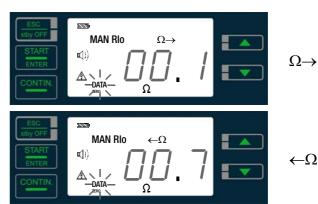
8.3 Taking Measurement Cables and Extension Cables into Account (up to 10 Ohm) – ZERO Function (Roffset)
