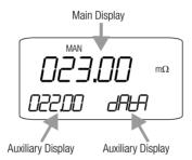
The main display appears immediately after the milliohmmeter is switched on, but the auxiliary displays have to be activated by pressing the DATAI CLEAR key.
