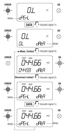
As long as the DATA function is active and all measurements are within the measuring range which has been automatically adjusted, the measuring ranges should not be changed manually.
