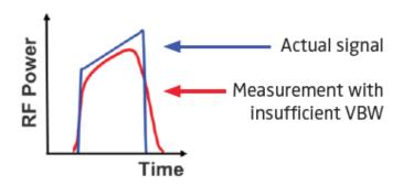
Video bandwidth (VBW) describes the ability of a power sensor to track peak (envelope) power. Insufficient VBW will result in errant envelope and average power measurements. The PMX40 offers the widest video bandwidth (195 MHz) making it ideal for measuring 80 MHz, 100 MHz, and 160 MHz channels
