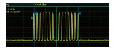
Proper design and operation of SSR systems is critical to the the safety and security of aviation. The PMX40 can be used to easily and accurately capture SSR waveforms. Markers enable measurements on specific portions of the waveform
