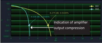
By comparing the peak-to-average power ratio, or crest factor (CF), of input and output signals of an RF transmission chain, engineers can assess circuit linearity. Additional insight can be provided with the PMX40 statistical mode **Complementary Cumulative Distribution Function** (CCDF) plot displaying the rate of occurrence of a specific CF. As an amplifier output compresses, the CF will reduce and the CCDF plot will move left.
